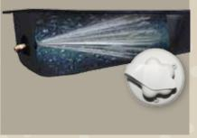
Cougar X-Lite comes outfitted with a black tank flush hook-up. This feature keeps the black tank clean and trouble free.
