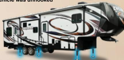
Utilizing a remote sensor located under the rear axle, the Level Up system accomplishes a level coach in seconds. This eliminates a time consuming and sometimes dirty task of manually leveling your coach.
