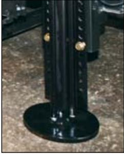
Standard Level-Up™ provides maximum stability with six heavy duty hydraulic jacks.
