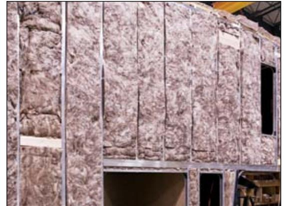
The coach and slide outs have aluminum wall studs and roof trusses positioned 16" on-centers, and the aluminum sub-floor joists are 14" on-center. Residential style high density wool insulation, in the side walls, is glued into place to prevent future settling. All spaces and voids are filled with wool insulation as well.
