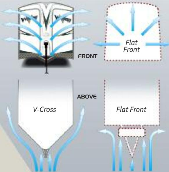
V-Cross design directs air flow around the sides of the trailer. Air impacts and scatters around and above flat front trailers.
