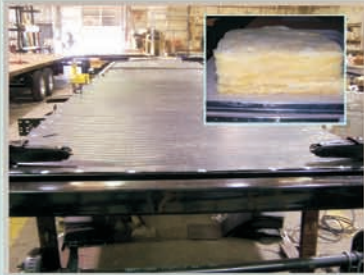
Fully Enclosed Front to Back Heated Insulated Underbelly Double Mountain Floor Insulation
