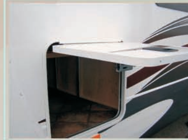
1" Thick Thermal Insulated Luggage Door Compartments
