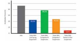
Compare acceleration forces experienced by an axle and trailer while traveling over railroad tracks at 30 MPH. The E-Z Flex® System provides up to an 80% reduction in forces on the trailer frame vs. a standard equalizer. E-Z Flex® significantly outperforms all other competitors in the same road test for a smoother, more protective ride for your trailer and cargo.
