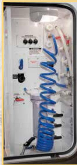
Docking Station includes outside shower, black tank flush, water filter, dump valves, and water tank fills for centralized convenience.
