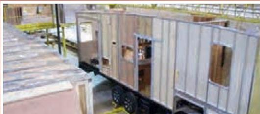
Aluminum studded sidewalls and roof trusses on 16" centers or less
