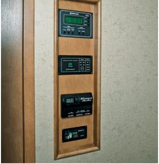
The **PowerLine® Energy Management System**, which prevents tripped campground circuits in periods of high demand, is part of the **OnePlace® Systems Center.**
