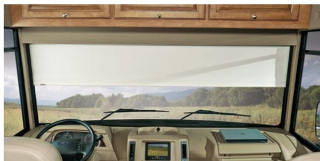
The **Powered Sunvisor** drops part way down at the press of a button to block the sun while you drive or all the way to the dash for privacy at the campsite.
