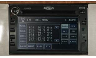
**RV Radio**<sup>®</sup> The innovative touch screen *RV Radio* features a CD player, MP3 input and doubles as the rearview monitor.
