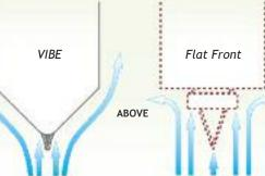
V-Design directs air flow around the sides of the trailer. Air impacts and scatters around and above flat front trailers.
