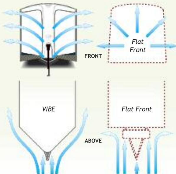
V-Design directs air flow around the sides of the trailer. Air impacts and scatters around and above flat front trailers.
