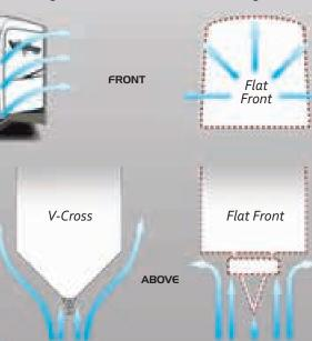
V-Cross design directs air flow around the sides of the trailer. Air impacts and scatters around and above flat front trailers.
