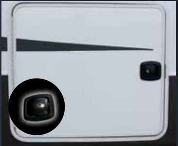
Bus-style Slam-Latch™ baggage doors are hinged on the side for easier access to the expansive pass-through storage. Metal catches slam and lock on metal strike plates, unlike the plastic latches used by the competition.
