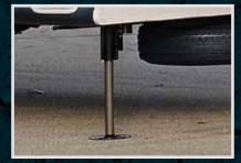
Wide stance power front jacks with quick release snap pins. (Optional hydraulic jacks shown)
