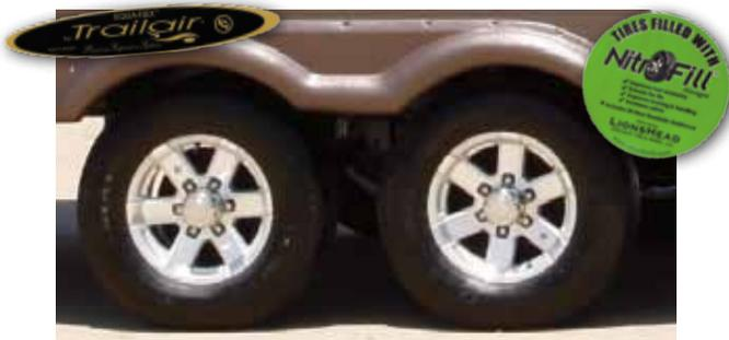
■ Nitrogen filled tires are standard on all Raven models. Also standard is a rubberized Equa-Flex Trailair® suspension system. Aluminum wheels are optional.
