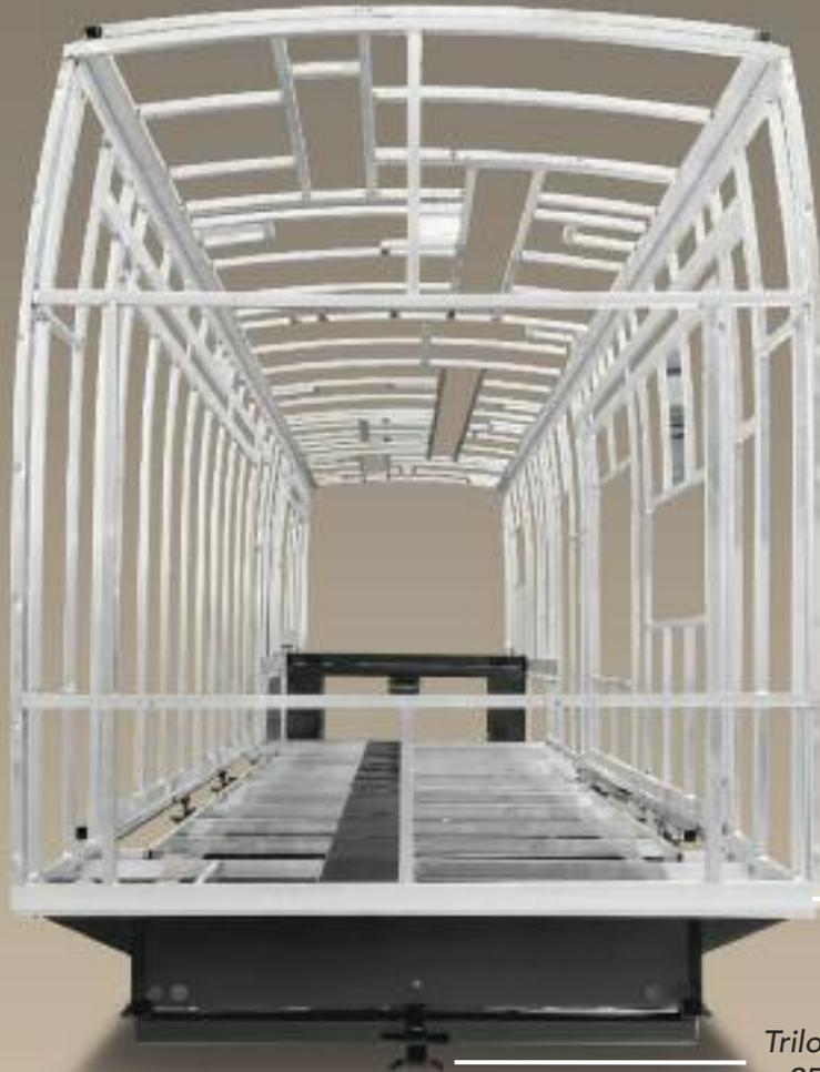
The roof structure is framed with 1-½" x 1-½" .062 gauge aluminum tubing and 1-½" x 1-½" .055 gauge P-tube. 1" x 1" solid wood is inserted into the P-tube for enhanced rigidity and improved screw retention.
