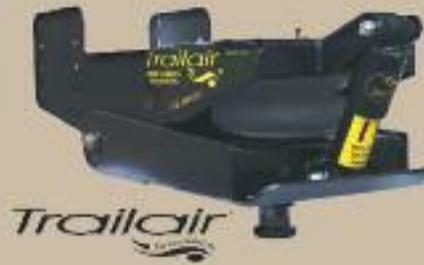
Trailair Air Ride Pin Box acts as a road impact buffer between the tow vehicle and the coach for smoother, more stabilized towing performance. The Trailair coupler's unique scissor action allows the air spring to absorb and dissipate these forces; the shock absorber handles the rebound effect.
