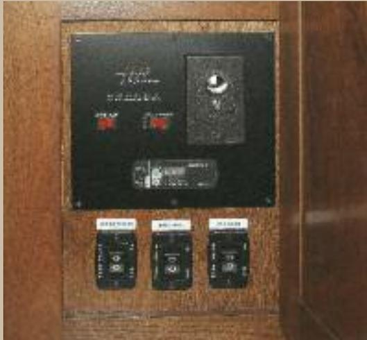
*This control panel is conveniently located near the entry, hidden behind a raised panel door. Controls: (3) slide out rooms, 1,000 watt inverter, (2) power awnings, monitor panel (LP, fresh, grey & black), water pump, water heater and TV booster.*
