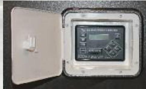
This electronic leveling control panel provides a one-touch auto-level feature. When it's time to depart, auto re-hitch memory restores the coach to the unhooked position. To retract, scroll to auto retract, press "enter" and in 20 seconds you're ready to hit the road.
