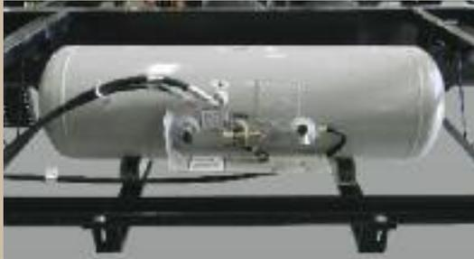
A 97 lb. LP tank is securely mounted between frame rails. Fill and vent valves, are accessed in the docking station. Trilogy is also equipped with a 20 lb. exchangeable auxiliary LP tank.
