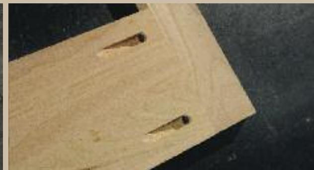
*Pocket screws for structural integrity*
