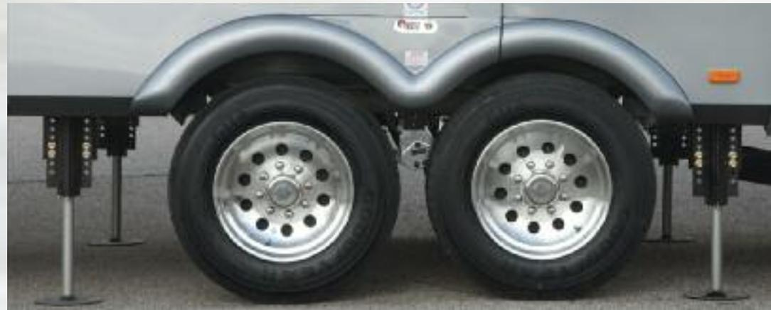
TrilogY is standard equipped with five Goodyear tires. Four are mounted on polished aluminum modular wheels. (Models 3800 RL and 3850 RL have 17.5" H-rated tires; Models 3650 RE and 3650 RL have 16" G-rated tires.)
