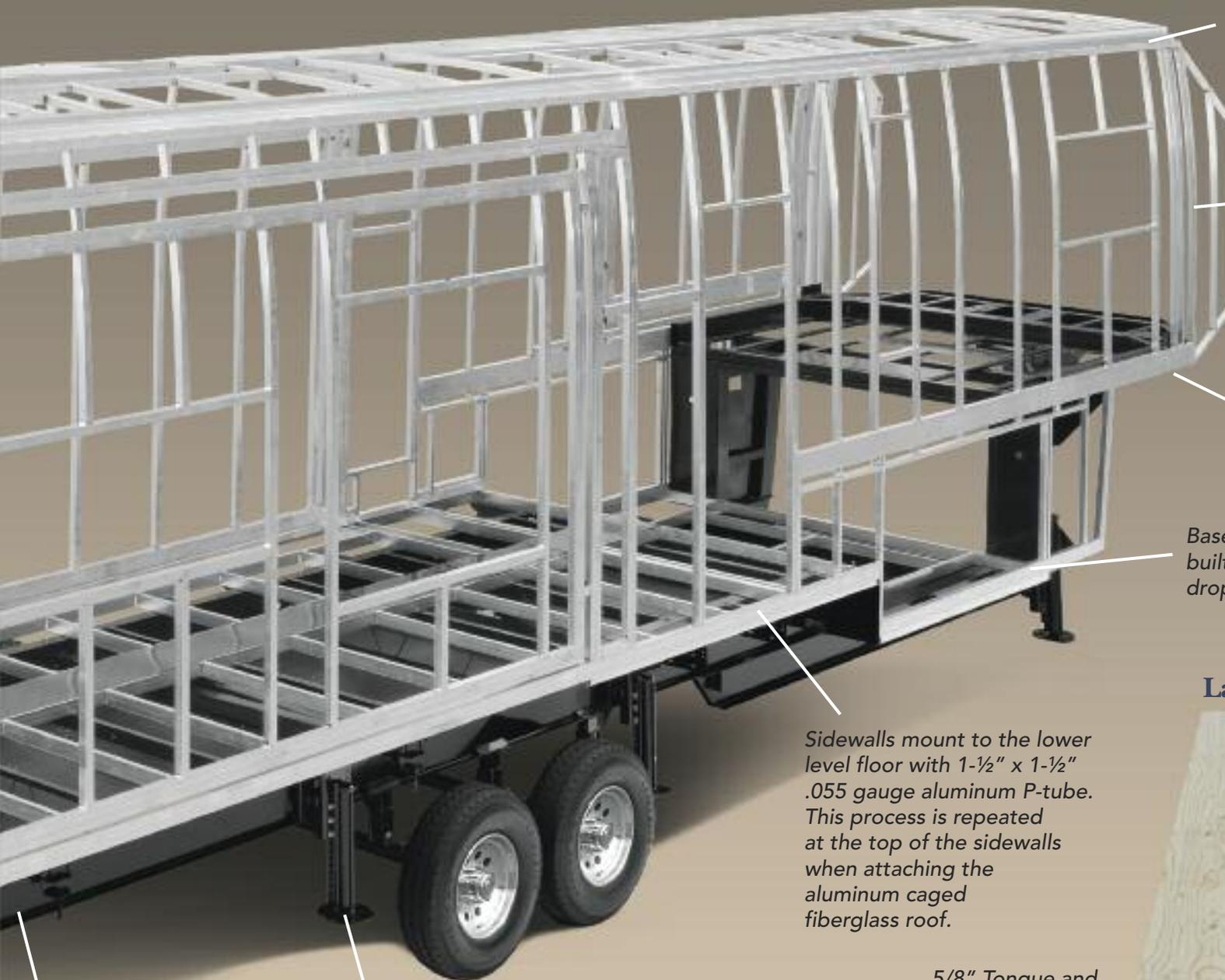
Sidewalls mount to the upper deck with 1-1/2" x 5" .188 gauge aluminum tubing.
