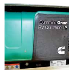
Propane Generator for charging your batteries, running the A/C or other 110 volt devices
