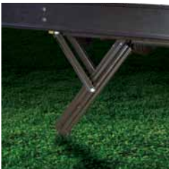
Stabilizer Jacks help keep your trailer stable on your campsite (Electric OPT)
