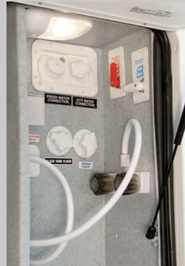
Exterior convenience center includes Within Reach water heater bypass valve, E-Z winterize valve, hot and cold exterior shower, black tank flush, 110V outlet plus cable and satellite hook-up.
