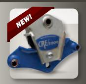
The MOR/ryde CRE 3000 suspension increases dynamic wheel travel by up to 3" by utilizing rubber and a unique travels lot to cushion shock. Increased travel means smoother towing and better protection from damaging road shock.
