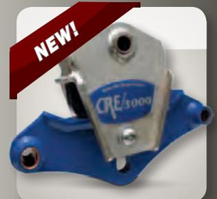
The MOR/ryde CRE 3000 suspension increases dynamic wheel travel by up to 3" by utilizing rubber and a unique travels lot to cushion shock. Increased travel means smoother towing and better protection from damaging road shock.
