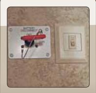
The battery disconnect is conveniently located in the pass through storage.
