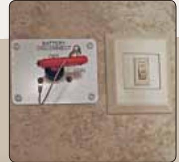
The battery disconnect is conveniently located in the pass through storage.
