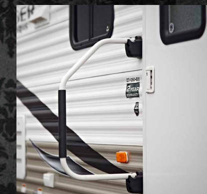
Swing out assist handle with 30° radius door
