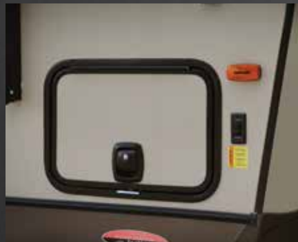
Slam Latches on Storage Doors
