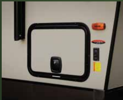
Slam Latches on Storage Doors
