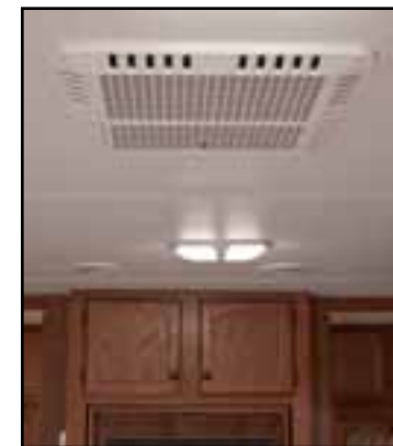
The ducted A/C distributes the cool air evenly throughout the travel trailer.
