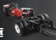
The Maxum chassis harnesses Winnebago Industries' SuperStructure® philosophy in tandem with the Freightliner XCL chassis. The Meridian 36M, 40U and 42E tag-axle ride on the Maxum chassis; its lowered rail design provides a lower center of gravity for improved ride and handling with up to 218 cubic feet of exterior storage. On the road, you'll get:
