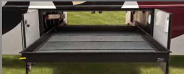
The lowered-rail design of our Maxum chassis has resulted in up to 218 cubic feet of exterior storage, which is incredibly easy to access with the available full-width **Slideout Storage Tray (36M, 40U, 42E)**.
