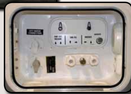
Exterior water center access.
