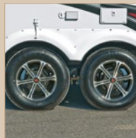
Cast aluminum wheels with radial tires
