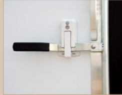
Security lock on ramp door
