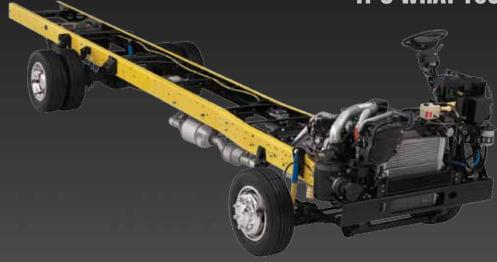
CHASSIS: Workhorse W20D chassis with a MaxxForce 6.4L V8 Diesel. 12-volt Alternator and In- Block, 6-Speed Allison MH-1000 Automatic Transmission. 19.5° Radial Tires. Stabil-ride(tm) Front and Rear Suspension. Hydraulic power 4-wheel anti-lock brakes. Bilstein(r) monotube gas-charged shocks absorbers. 5,000 lb Trailer Hitch. Fully Automatic 4 Point Leveling Jacks and more.
