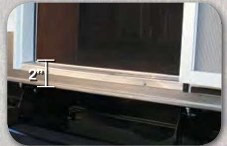
This 2" thick floor has a full R-8 insulation, to help keep your trailer nice and comfortable
