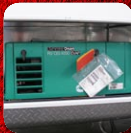
4.0k Built-In Onan Generator
