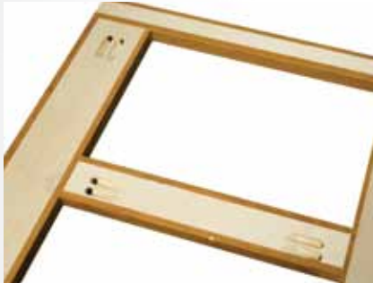
Glued and screwed wood cabinetry
