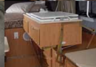
Swing down galley (Except LTDs)
