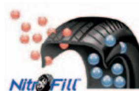
Our wheels feature nitrogen-filled 10-ply E-rated radial tires standard across the line. Nitrogen reduces deterioration and helps maintain proper PSI over time.
