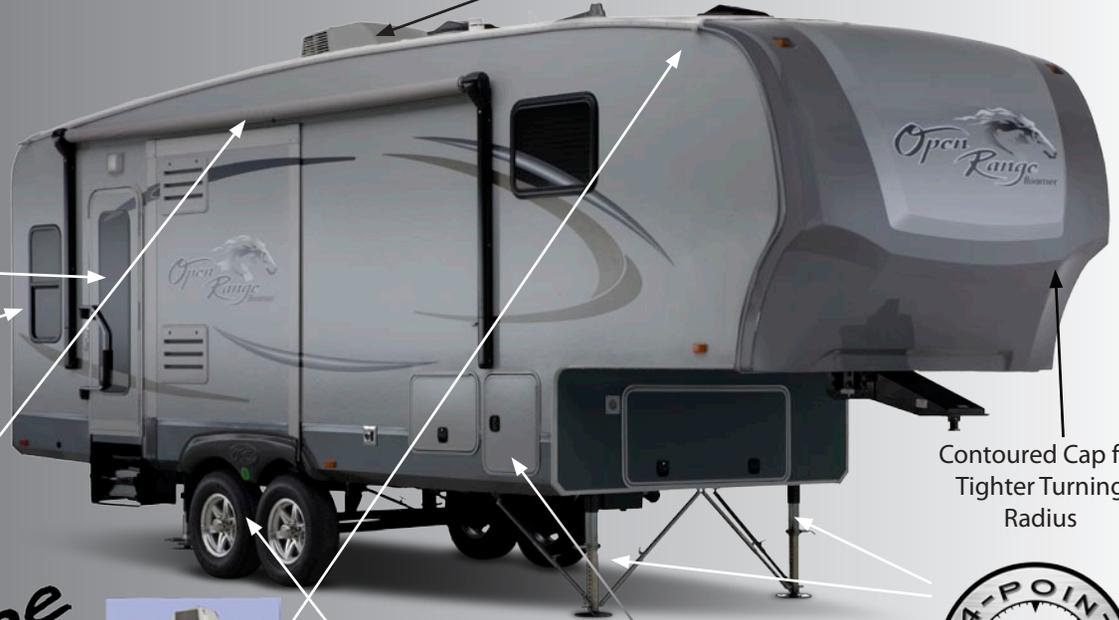
Contoured Cap for Tighter Turning Radius
