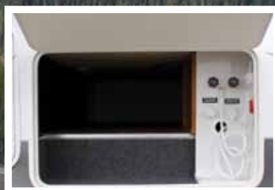
Docking Station with Quick Winterizing Feature. (FW's Only)
