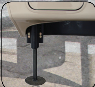
Six Point Automatic Hydraulic Leveling
