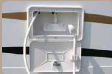
**Exterior shower** comes equipped with a fixed shower head and access to both hot and cold water.
