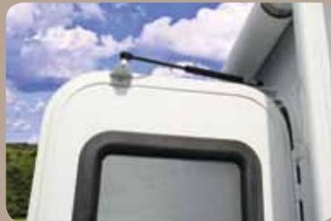
**Gas struts** eliminate the concerns of replacing brittle plastic door catches.
