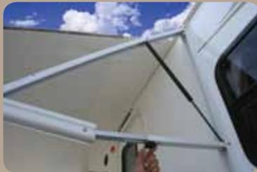
**Electric awning** with adjustable arms makes it easy to extend/retract the awning as well as adjust the ends for water run-off.
