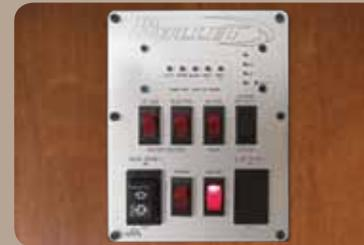
**Monitor Panel** provides a central location for patio awning, slideout and light switches
