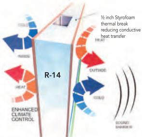
Canyon Trail's unique sidewall construction used on all our products is constructed with welded aluminum, solid 2" wall of two pound density polystyrene.
