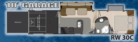
Overall Length: 37' 9" Pin to Bumper: 33' 9" Dry: 11,950 GVWR: 14,000 Hitch: 2,900
