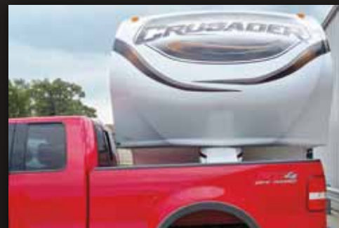
JPER TURN® Front Cap Has 88 Degree Turning Radius
