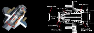
E-Z lube axles allow you to repack your wheel bearings quickly and easily without disassembly.
