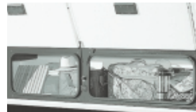
Our EZ Store™ Storage System was developed using a rack and pinion system to give you the utmost ease in accessing your stored gear below. (Available on SL Model 31W only)
