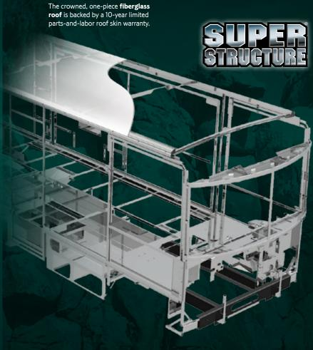
Metal substructures secure cabinets and appliances to add safety and stability.
