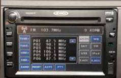
**RV Radio** AM/FM stereo, CD player, weather band and remote are all part of the RV Radio. The 6.5" touch screen also displays the rearview and available sideview camera images.
