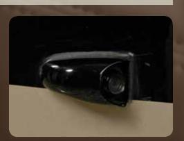
**Sideview Cameras** Available sideview cameras activate with the turn signals and display on the in-dash screen to assist with maneuverability and visibility.
