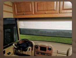
**Front Shade** The MCD American Duo front roller shade is a powered visor and has both a light-filtering shade and a blackout shade.
